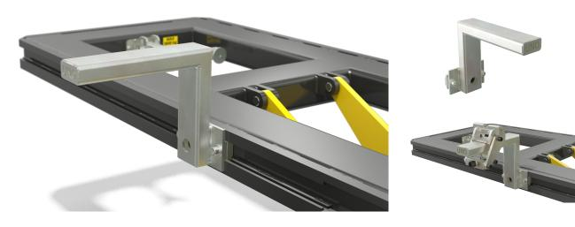
The UnoLiner B10 Bench Adapter is the standard yet versatile bench adapter for all UnoLiner bench frame machines. Each UnoLiner Straightening Bench Set comes equipped with four of these bench adapters, which can be placed all around the bench frame with its unique Quick Lock one-bolt locking system. The B10 supports all types of UnoLiner chassis clamps.
